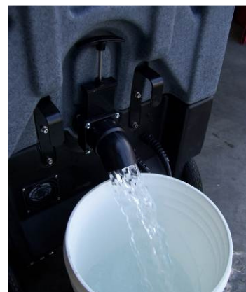
Drain water from Recovery Tank
