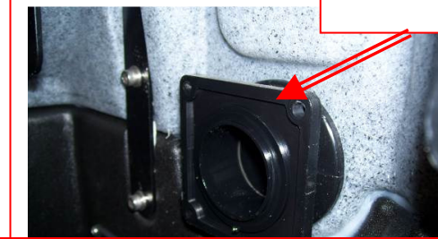
Unless damaged or leaking between tank and flange, the flange fitting does not have to be removed
