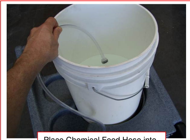
Place Chemical Feed Hose into Rinse Solution
